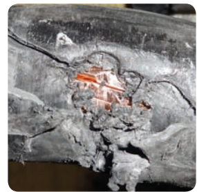
Major cable damage caused by thread contact
